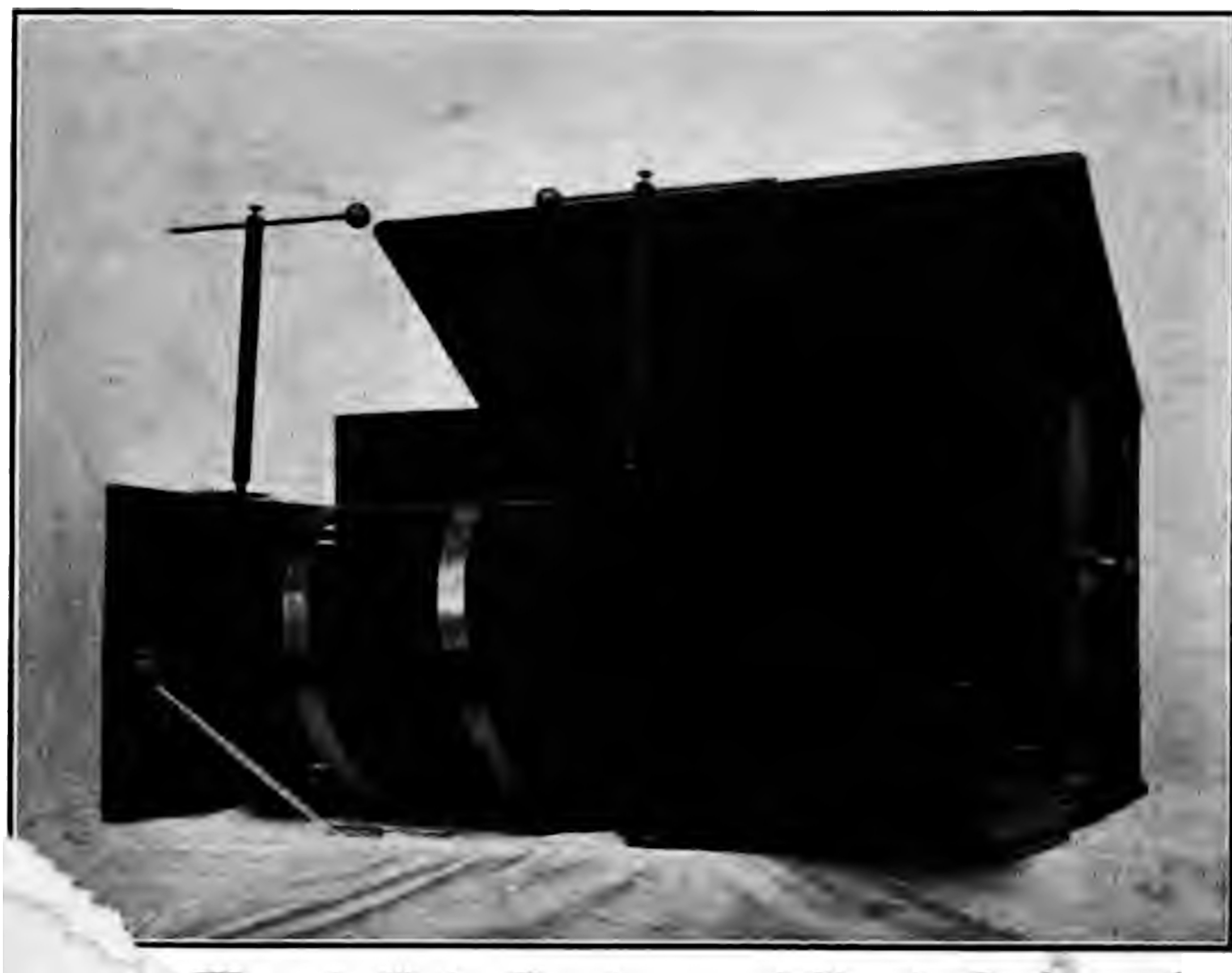
III. — Oscillation Transformer and Glass for Condenser of 12" Coil.
