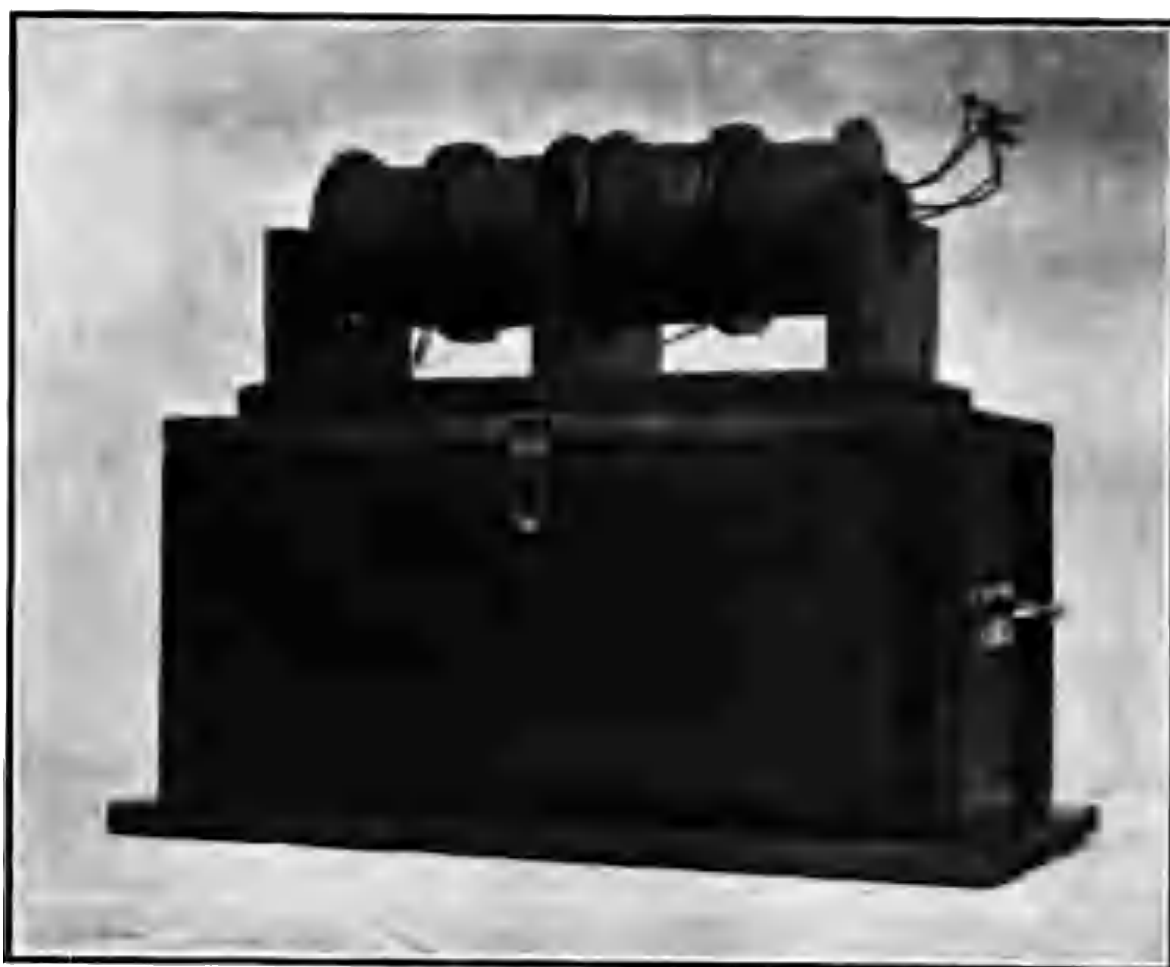
PLATE II. — Transformer for 12" Apparatus.
